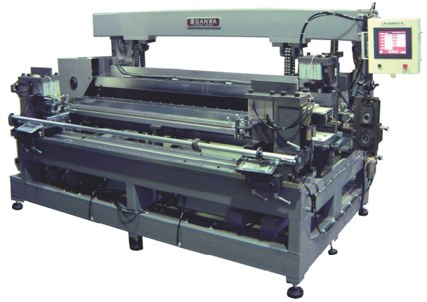
Fig. 10 – Fully automatic CNC type crimping /weaving line .
