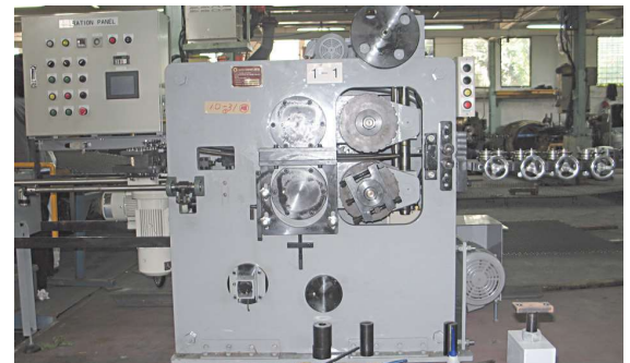
Fig. 8 — PC-1 model for wires 1 to 4 mm (top) and PC-40 model for wires 1 to 12 mm (bottom).
